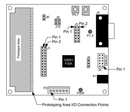
Figure 4. C8051F330 Target Board
