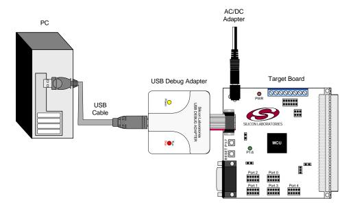
Figure 1. Hardware Setup Using a USB Debug Adapter
